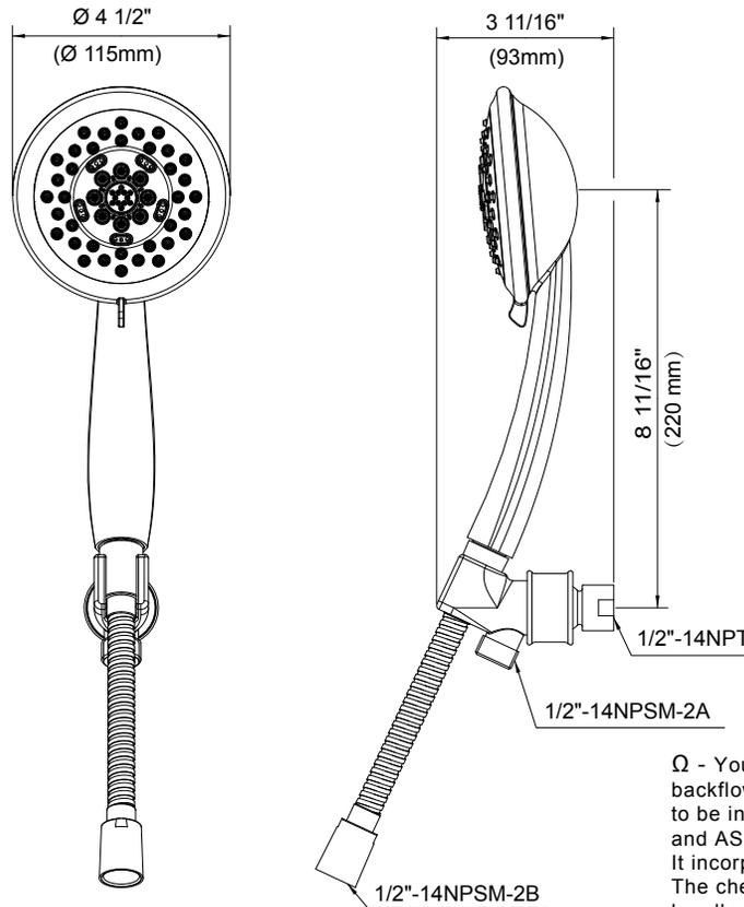
$\Omega$  - Your Danze handshower kit incorporates a backflow protection system that has been tested to be in compliance with ASME A112.18.3 and ASSME A112.18.1/CSA B125.1. It incorporates two certified check valves in series. The check valves are located in the handshower handle, and either the supply mount or the showerarm mount outlet.
