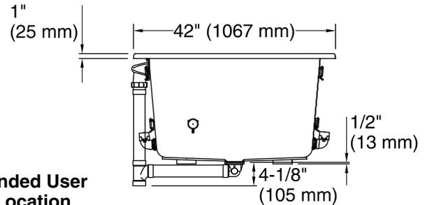
No change in measurements if connected with required drain illustrated. (K-7272)
