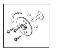
6 Snap on the remaining rose. Slide the remaining knob or lever onto the spindle and secure with set screw.
