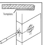
2 Caution: Re-check bore hole locations before drilling. Drill the face bore and edge bore as indicated on template.
