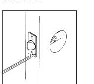
Chisel out the area marked in step 3 to a depth of 5/32" or until faceplate is flush with door edge. You may now proceed to Strike Installation.
