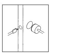
Insert the latch into the edge of the door. Trace an outline of the faceplate onto the door edge. Mark and drill screw hole centers with 1/8" drill.
