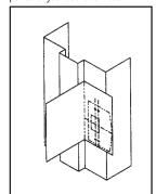
Align the strike and trace outline onto the door frame using mounting screw marks for location.
