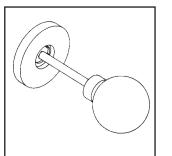
Slide the remaining backplate onto the spindle. Rotate the backplate to take up any slack. Mark and drill pilot holes. Tighten screws.
