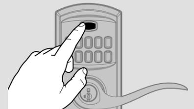
**E** Enter a Programming Code. It must be between 4 and 8 digits. **The Programming Code cannot be the same as any user code.**
