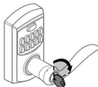
**b** To remove the key, turn the key back to the vertical position.
