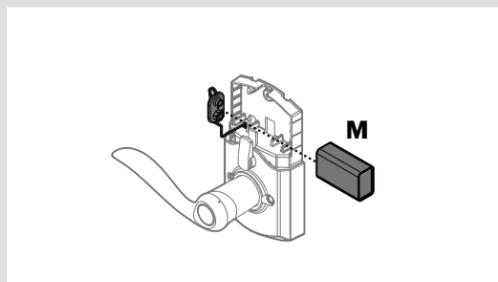
**C** Secure battery into interior assembly.
