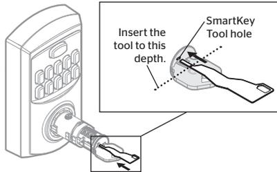
**c** Fully insert your new key into the lock and turn it 180° counterclockwise. Next, turn the key 90° back to the starting position, then remove it.
