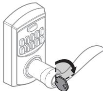
**c** Secure the lever by tightening the pre-installed set screw.
