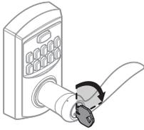
**b** Loosen the pre-installed set screw.
