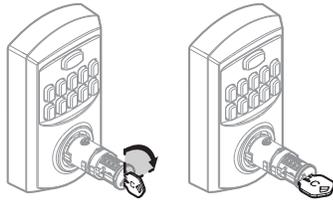
**b** Insert the SmartKey tool fully and firmly into the SmartKey hole, then remove the SmartKey tool and current key.
