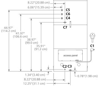
BS\*- Base stand sold separately; measurements shown are with base stand legs at lowest position. See dispenser detail sheet, form# 6675, for counter cut outs.
