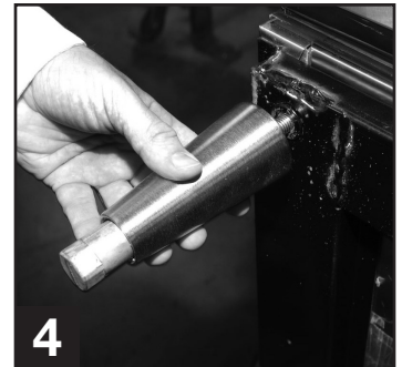
4 Thread leg into cabinet bottom frame rail.
