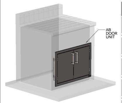
**AB - ACCESS DOOR TYPICAL INSTALLATION**
