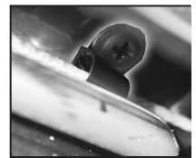
P-Clip keeps cord in-place (prevents cord damage).
