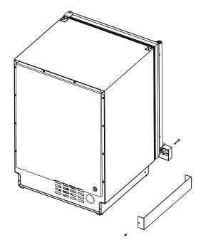
3. Align front hole with hole in shell accessory, hole in base, and hole in grille. Tighten screw.
