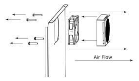
13. Remove and replace fan. Take special care to properly route fan wire.
