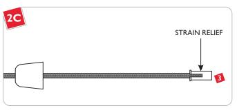
Insert the coaxial cable through the flared end of the strain relief.
