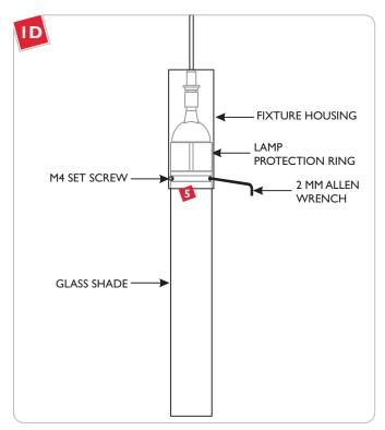
Push the grooved section of the acrylic shade into the fixture housing and tighten the three M4 set screws with the provided 2MM Allen wrench to secure the acrylic shade in place.
