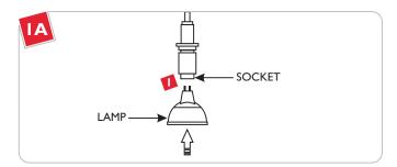
**NOTE:** To reduce the risk of a burn or electric shock during relamping, disconnect the power to the fixture.
