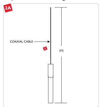
Cut the coaxial cable to the desired length with a sharp cutter. The overall fixture height (H) is measured from bottom of the acrylic shade to end of the coaxial cable.
