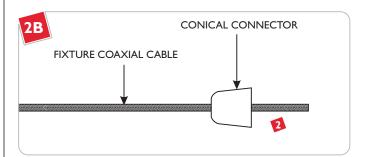
1 Insert the fixture coaxial cable through the conical connector.
