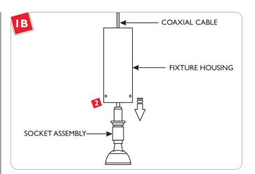
Feed the fixture coaxial cable through the fixture housing. Slide the fixture housing down the cord and rest it onto the socket assembly.
