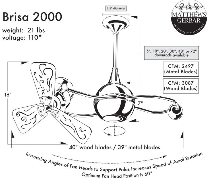
The Brisa can be mounted with any one of the following downrod lengths: 5, 10, 20, 30, 48 or 72".
