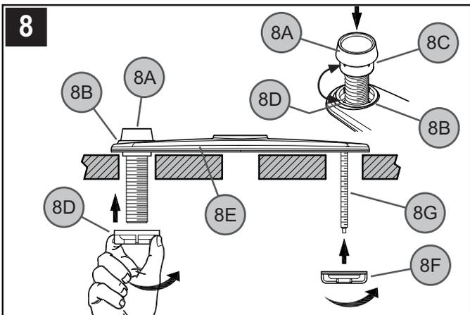
Insert Hose Guide (8A) into the side hole in the Deckplate (8B) and onto the sink hole. Align the hose guide Tabs (8C) to those in the Deckplate Hole (8D). From underneath sink, secure the Hose Guide (8A) by screwing the Plastic Locknut (8D). Secure Deckplate (8E) by screwing Wing Nut (8F) to Mounting Post (8G). Hand tighten. **Caution: do not over-tighten.** Remove any excess putty from around the outside edge of Deckplate (8E).
