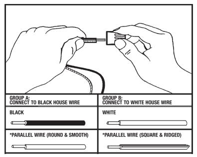
**A.** Take note of the color of the wire(s) on your fixture. Identify which group your fixture wire(s) falls into and connect the wires according to the directions below:
