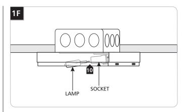
**CAUTION:** To reduce the risk of a burn or electric shock during relamping, disconnect the power to the fixture.
