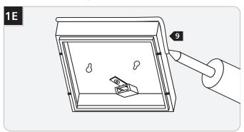
For wet location installation, caulk around the mounting base with waterproof construction sealant.
