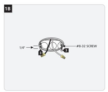
Thread (NOT COMPLETELY) the two #8-32 screws into the electrical box holes leaving 1/4" of them exposed.
