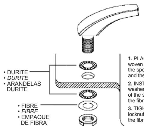
1. PLACE first DURITE (coarse woven abrasive) washer between the spout (of offset spout body) and the top of the sink.
