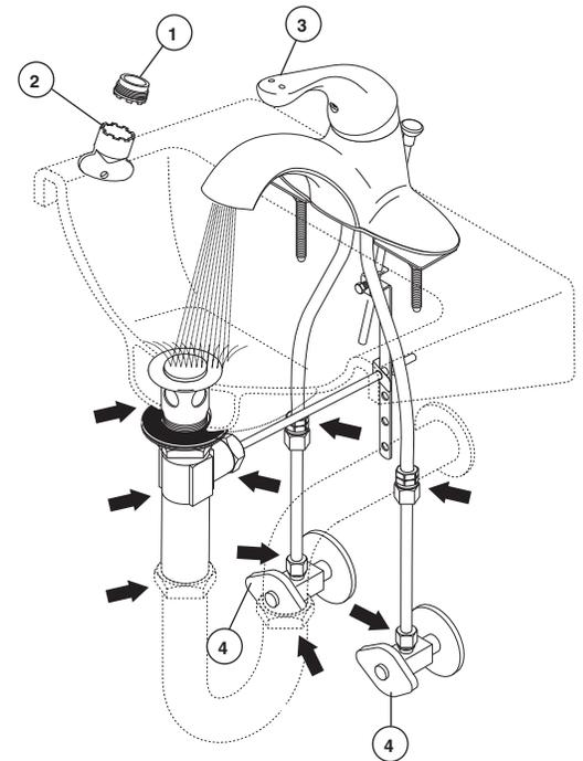
Remove aerator (1) using supplied wrench (2) and move faucet handle (3) to the full on mixed position. Turn on hot and cold water supplies (4) and flush water lines for one minute. **Important: This flushes away any debris that could cause damage to internal parts.** Reinstall aerator. Check all connections at arrows for leaks. Re-tighten if necessary, but do not overtighten.
