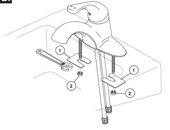
**A.** Position faucet (1) and gasket (2) on sink. *Option: If sink is uneven, use silicone under the gasket.*
