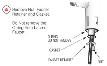
Install Faucet with O-ring **FAUCET** into the center hole in deck or lavatory — 1-3/16" (30 mm) min. hole required. Note: If installing the Faucet on a three (3) hole sink, a Trim Plate should be installed at this time. ~0-RING CENTER HOLE IN DECK OR LAVATORY Slide Gasket over Flex Hose(s) and secure with Faucet Retainer and Nut.
