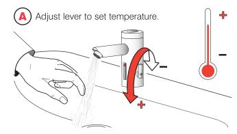
**B Optional** — To fix temperature, set lever to the desired position, then remove lever and plug hole with Cap.
