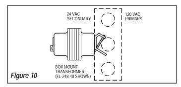
This type of Transformer is designed to be mounted on a metal electrical junction box (supplied by others). ("J" box should be mounted inside chase wall or above ceiling.) Install Transformer within 50 feet (15.24 meters) of Faucet. 18 gauge wire is recommended.
