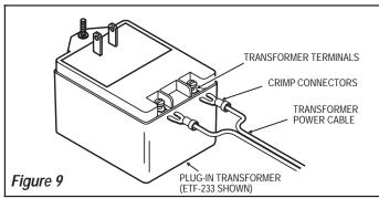
Install Crimp Connectors to opposite end of Transformer Power Cable and connect Power Cable ends to Transformer Terminals as shown in Figure 9.
