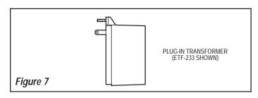
This type of Transformer is designed to be plugged into a 120 VAC wall receptacle. The Transformer is supplied with a 10 foot Cable; however, this Cable can and should be shortened to meet installation requirements.
