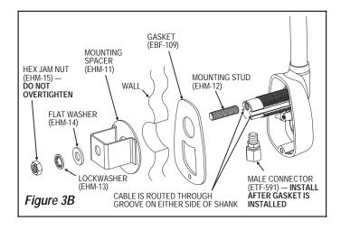
**Note:** Sloan Valve Company does NOT supply hardware necessary for mounting the faucet on surfaces thicker than 1" (25 mm) thick.
