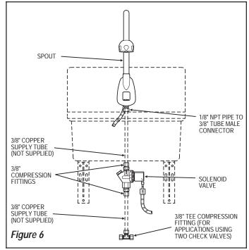
Thread Male Connector into inlet hole at bottom of Spout Shank; tighten securely to prevent leaks.
