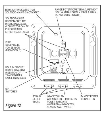
Open Supply Stops. With Spray Head removed, activate Faucet for 30 seconds by placing hands in front of Sensor. The Solenoid Valve should "click" and water should flow from the Spout. If this does not occur, refer to the Troubleshooting section of this instruction manual.
