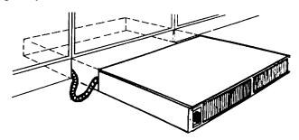
Run electrical power cable to installation location. Provide two feet of slack to allow heater to be pulled out far enough to remove top cover for cleaning or servicing.
