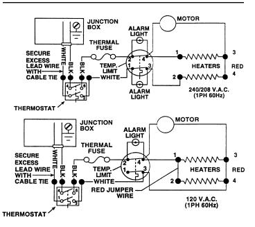
If a 120 V.A.C. circuit is to be used, make wiring changes as follows:
