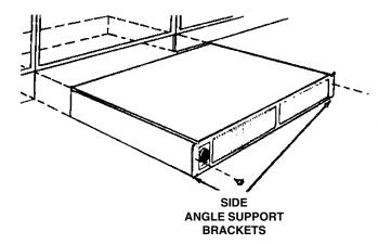
The unit will be secured in place with screws through the side angle support brackets. Provide adequate material behind side angle support for secure mounting.
