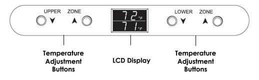
You may adjust the temperature of the wine cooler using the front panel controls. The temperature displayed will be in Fahrenheit. This wine cooler is a dual zone with two separate temperature regions. The Upper Zone range is 45°F to 54°F and the Lower Zone is 54°F to 64°. Whether your wine cooler can reach the actual set temperature depends on the ambient environmental conditions.
