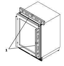
2. If the unit is not level, adjust the legs on the corners of the unit as necessary.
