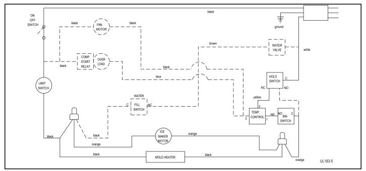
Figure 2. Harvest-1 Cycle (Hold Switch in Normal Position)
