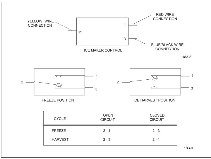
Figure 5. Temperature Controls - Manual Defrost Ice Makers
