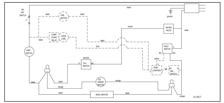
Figure 4. Water Fill Cycle
