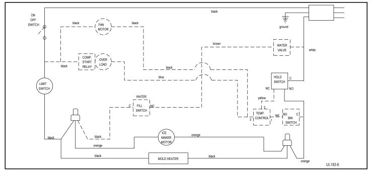
Figure 3. Harvest-2 Cycle (Hold Switch in Switched Position)
