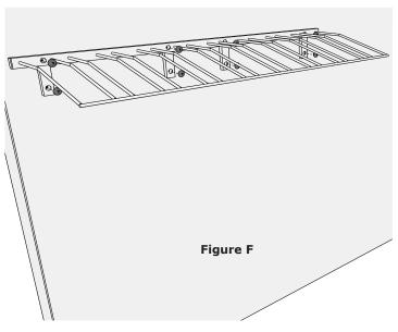
\*Alternate Installation\* Attaching to FCF-HD - Place the rack against the FCF-HD in the position where it is to be installed and ensure that it is horizontal using a level. To secure the rack, use the Self Drilling Screws provided with the FCF-HD and fasten the rack through each of the 8 mounting holes.
