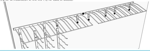
1. **Mark the mounting hole locations** - Position the rack on the wall where it is to be installed and use a level to ensure the rack is perfectly horizontal. Using a pencil, mark all 8 mounting hole locations (Figure A) and set the rack aside.
