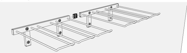
1. **Mark the mounting hole locations** - Position the rack on the wall where it is to be installed. Make sure there is adequate space underneath the rack for your stemware to hang. Use a level to ensure the rack is perfectly horizontal. Using a pencil, mark all 4 mounting hole locations (Figure A) and set the rack aside.
