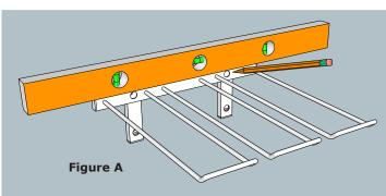
Note: If a marked hole location is over a stud, the Spiral Drywall Anchors or Toggle Bolts should not be used. Drill a pilot hole in the stud with a 3/32 inch (2.4mm) drill bit and use the extra Screws supplied to fasten directly into the stud.
