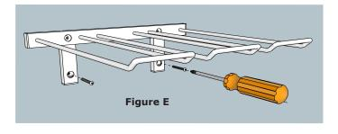
\*Alternate Installation\* Attaching to FCF-HD - Place the rack against the FCF-HD in the position where it is to be installed and ensure that it is horizontal using a level. To secure the rack, use the Self Drilling Screws provided with the FCF-HD and fasten the rack through each of the 4 mounting holes.
